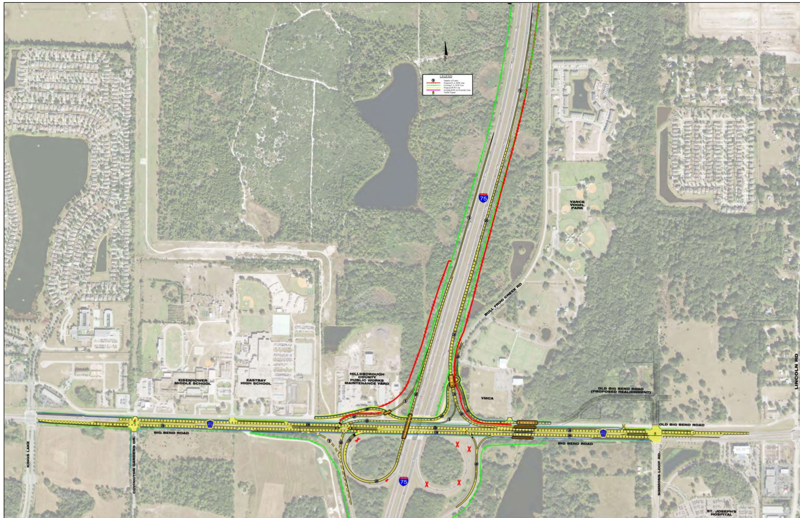
Figure 3A – Proposed Lane Geometry and Traffic Control (Sheet 1 of 4: I-75/Big Bend Road Interchange – Overview)
