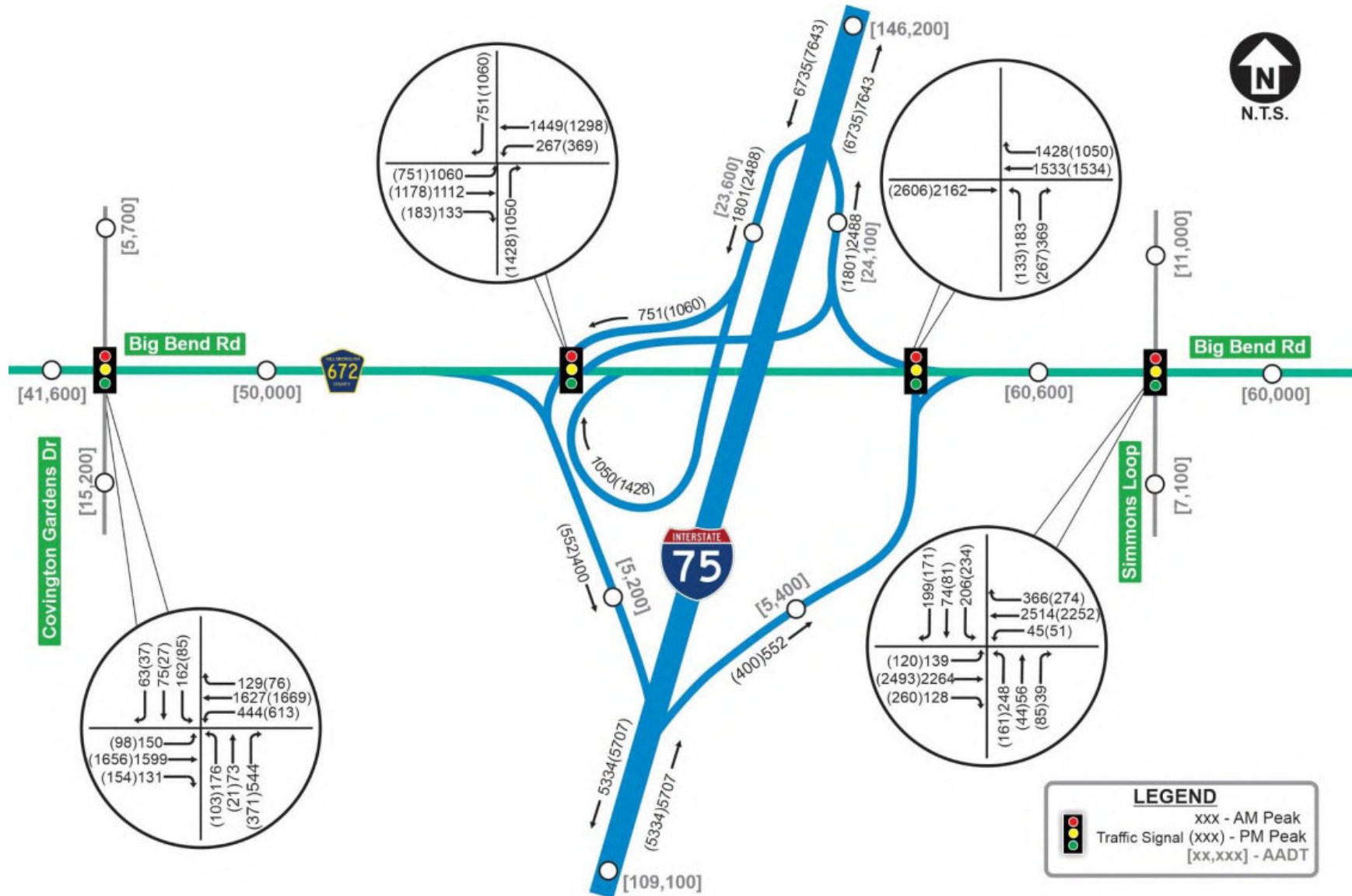
Figure 10 – Opening Year (2025) Build Alternative AADT, AM and PM Peak Hour Turning Movement Volumes
